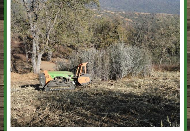
Through a grant from Cal Fire Tulare County RCD was able to acquire and utilize a cutting-edge masticator, the Green Climber LV600, which is a new tool in the Sierra. This masticator requires up to 90% less fuel to operate and transport compared with traditional larger machines. It is controlled remotely providing an unparalled degree of operator safety, and has been demonstrated to be effective on slopes up to 60 degrees.
